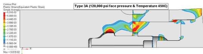
Figure 3. New high-pressure dummy block under 84 kg/mm<sup>2</sup> (120,000 psi) specific pressure.
