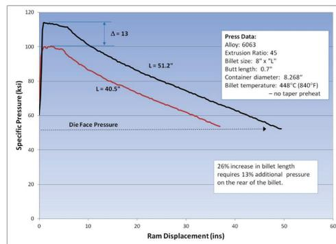
Figure 1. Specific extrusion pressure for two different billet lengths.
