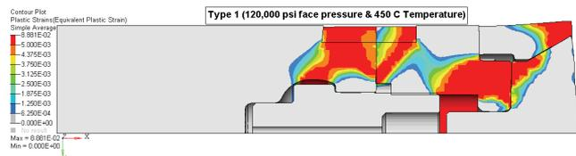
Figure 2. A dummy block under 84 kg/mm<sup>2</sup> (120,000 psi) specific extrusion pressure.
