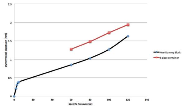
Figure 5. The interaction of new high-pressure dummy block and three-piece container.
