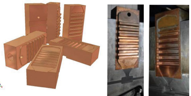
Figure 8 - Copper chill vents require no water cooling and no ejector pin.
