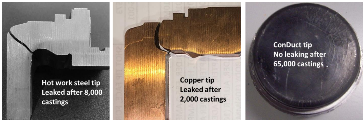
Figure 2: Water-cooled plunger tips of the same size made of different materials (hot work tool steel, Copper alloy and ConDuct). Failed tips were sectioned for inspection study.
