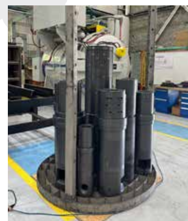
H-13 tooling being loaded for processing in the new nitrocarburizing system.
