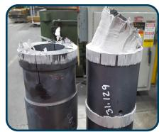
Through the ongoing development of metal treatment and casting technologies, the quality of alumimum alloy billets is constantly improving. The outer skin of the billet, however, is inevitably oxidized, and often also marred by surface impurities and minor inclusions.
