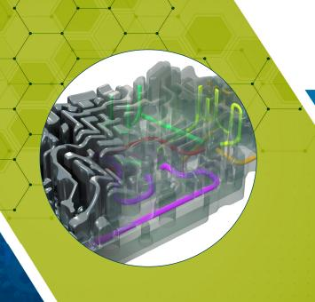
Additive manufacturing can thermally improve die casting conditions, resulting in reduced cycle times and extended tooling life. This is accomplished by conformal cooling channels which were impossible with conventional manufacturing processes.
