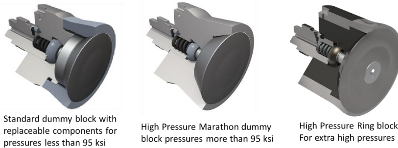
Figure 10 – Different dummy blocks designed for different face pressures
