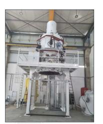
Castool has dedicated heat treatment and nitride facilities in Canada, Thailand and Morocco. Each has 12-bar vacuum heat treatment furnaces capable of heat treating 15,000 lbs and vertical tubes up to 65" in length. We can nitride virtually any heat treated tool also in vacuum.
