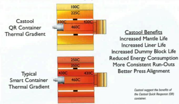
The thermal mass of the container is so much greater than that of the die, so that as soon as the die is clamped onto the container liner, the face of the die assumes the temperature of the exit end of the container until the run is completed.
