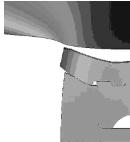
Figure 7. A cross-sectional view of the deflection of dummy block and container. Radial distortion has been exaggerated for emphasis.
