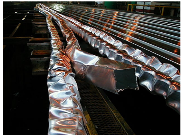
Figure 1. Extrusions from the first two billets must be scrapped before acceptable production is achieved
