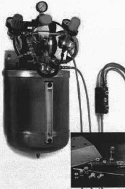
Castool's liquid boron-nitride lubrication system
