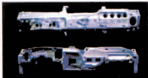
Figure 1: Die cast auto dashboard.
